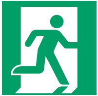
Escape route / emergency exit (right)
