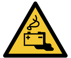
Warning of danger from charging batteries
