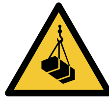
Suspended load warning
